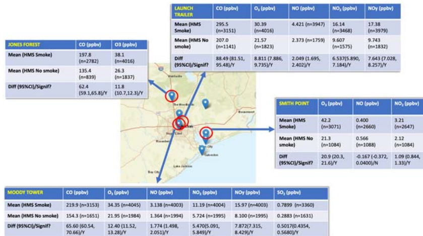
Figure 1. Map of selected surface air quality monitoring sites in HGB. Tables show concentrations of species measured at each circled site, divided into HMS-smoke and HMS-no smoke categories.
