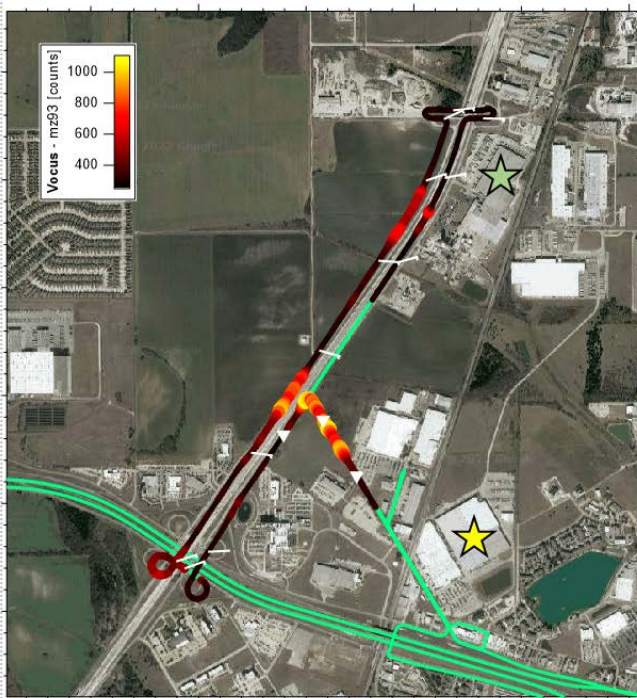
Figure 4; The route of the AML is depicted at left colored by the m/z93 (toluene) intensity as measured by VOCUS and the time series of m/z 93 (toluene) is depicted at right.
