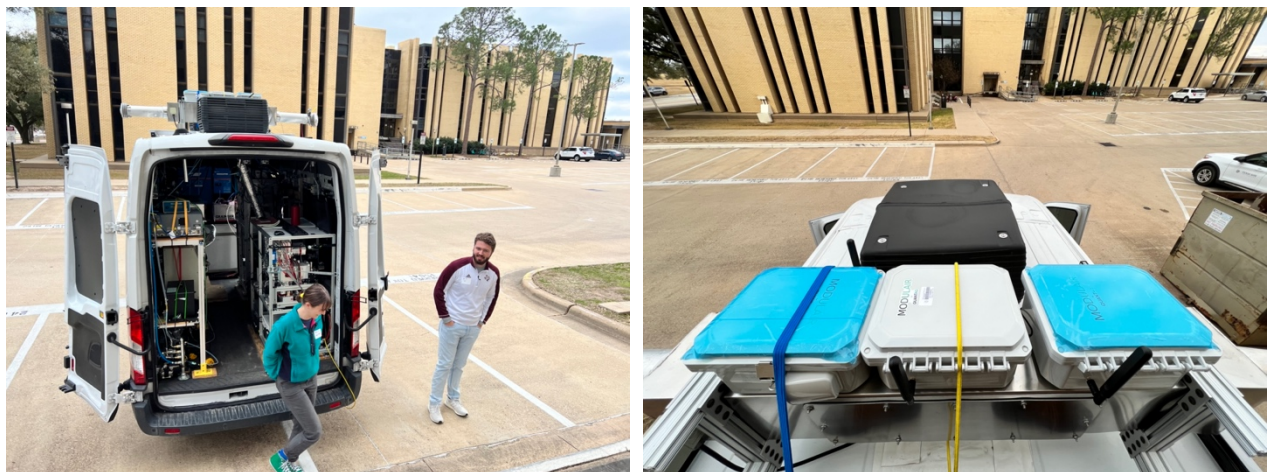
Figure 2. Exterior and roof top (with three air sensors) view of the mobile laboratory
