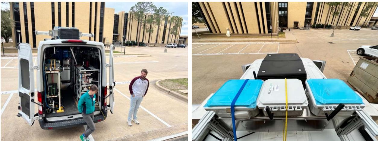
**Figure 22-020-9.** Exterior and roof top (with three air sensors) view of the mobile laboratory
